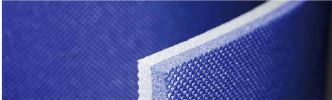
LDPE foams are semi-rigid. In order to impart more softness and resiliency to LDPE foams polar copolymers in the range between 10 % - 50 % are often added as part of the formulation. Suitable polar copolymers are poly butyl acrylat, poly methyl acrylat, poly ethyl acrylat and poly vinyl acetat. In order to be fit for use in their specific applications and markets, such as automotive, building and aerospace, excellent low temperature properties are often very important.
