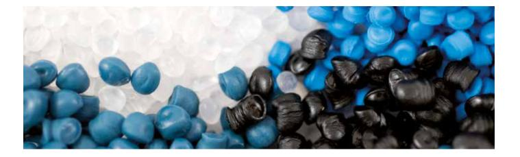
Commercial polyamides such as PA-6 and PA-66 are generally regarded as tough and ductile materials since they exhibit high tensile elongation to break and high drop weight impact strengths. They become even tougher after equilibration with ambient humidity due to the plasticization effect of the absorbed water.
